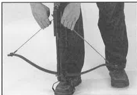
7. With foot firmly grounded in stirrup for stability, pull the stringer upwards and lock securely into the trigger mechanism. Make sure to engage "Safety".
