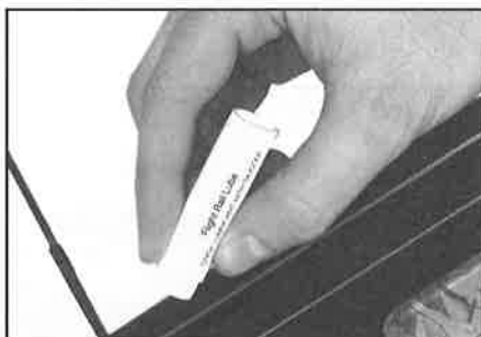
28. Before using, lubricate the string serving and rail. Failure to do so will result in the string serving burning and wearing out prematurely. We recommend applying the wax every 10 to 15 shots.
