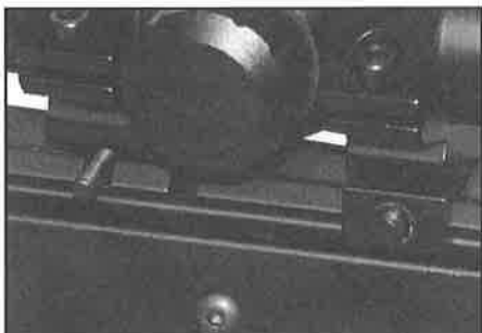
25. Slide in each of the mounting brackets in the desired position on the weaver style sight base.
