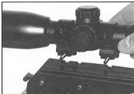
24. Align the scope mount with the slots on the weaver style sight base.
