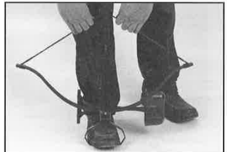
19. With foot firmly grounded in stirrup for stability, pull the string upwards and lock securely into the trigger mechanism. Make sure to engage "Safety".
