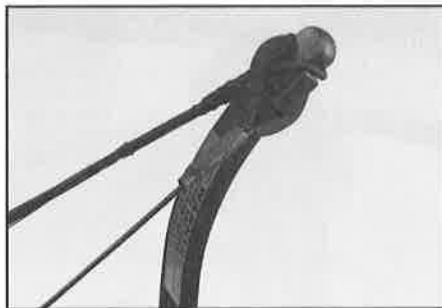
8. Attach the string loop to each limb tip by inserting through/under the stringer loop. Be sure that the crossbow stringer is fully looped over both sides of plastic tip (as shown).
